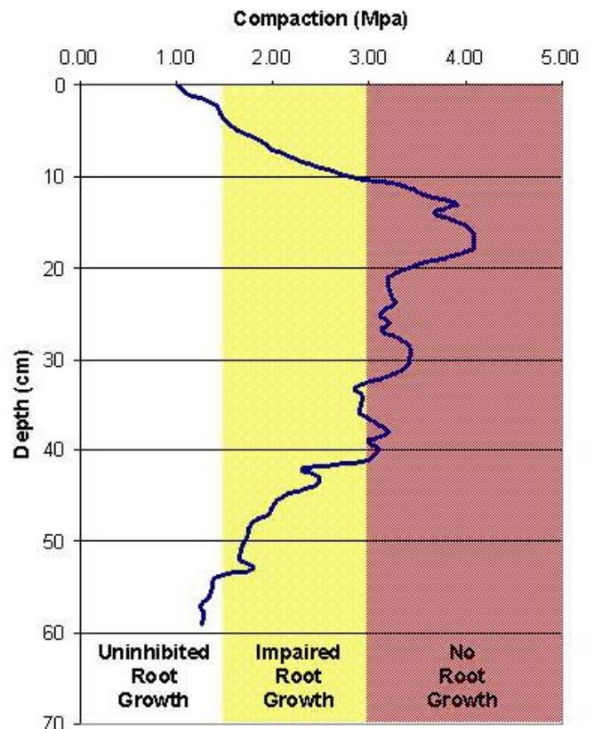
reduced relative to typical native soils. Pitt et al. (1999), found that the infiltration rate averaged 13 inches/hour and 1.4 inches/hour, respectively, for non-compacted and compacted sandy soils. For dry clayey soils, the infiltration rate averaged 9.8 inches/hour and 0.2 inches/hour, respectively, for non-compacted and compacted soils.
